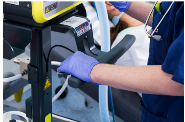
The auto-lock brake locks the trolley wheels as soon as you let go of the handle
