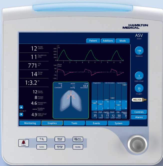
Blue alarm lamp on top of ventilator lights to indicate heliox is being administered.
